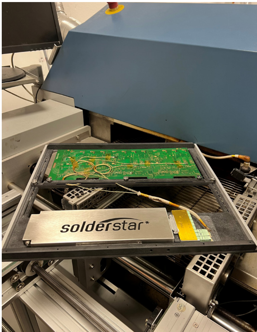
■ Profiling carrier installed inside a vacuum reflow oven to record real board temperatures and vacuum behaviour during the process cycle.
